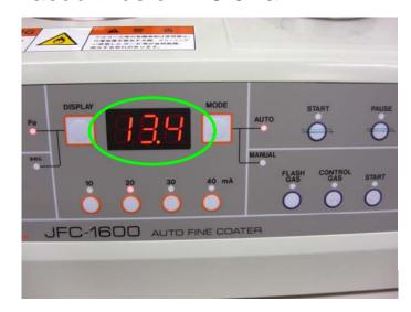
5. Switch to [sec] with pressing [DISPLAY], and set time/current.
